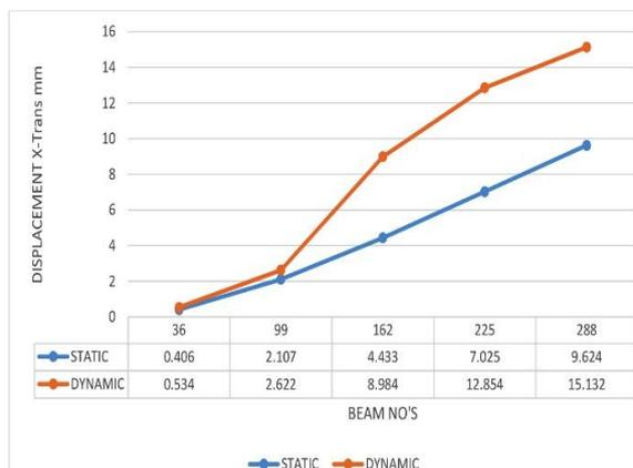
Graph 8. Static & dynamic analysis of Displacement in SMRF
