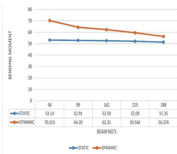
Graph 7. Static & dynamic analysis of Bending Moment in SMRF
