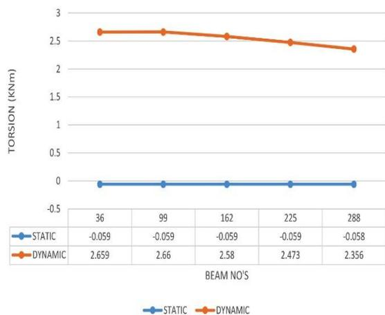
Graph 6. Static & dynamic analysis of Torsion in SMRF
