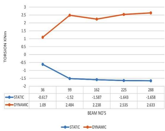
Graph 2. static & dynamic analysis of Torsion in OMRF
