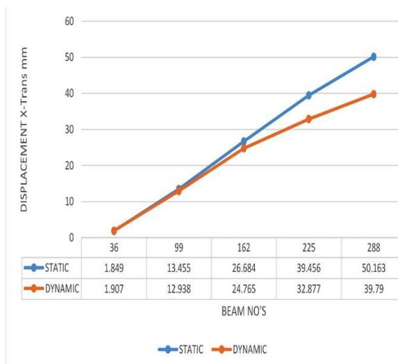
Graph 4. static & dynamic analysis of Displacement in OMRF
